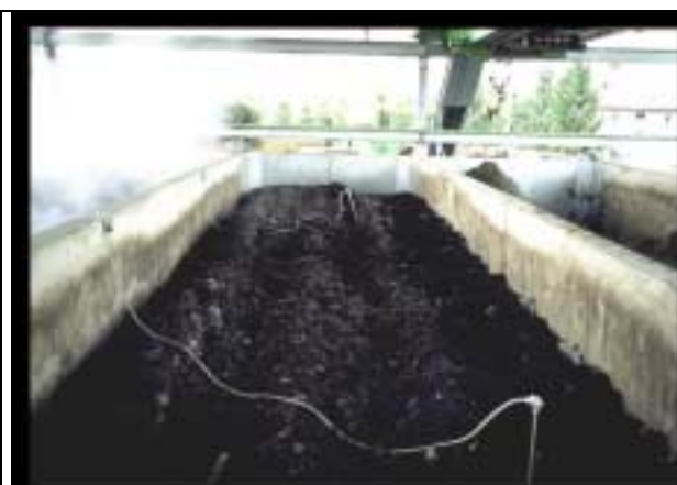
Composting in box (System COMPAG)
