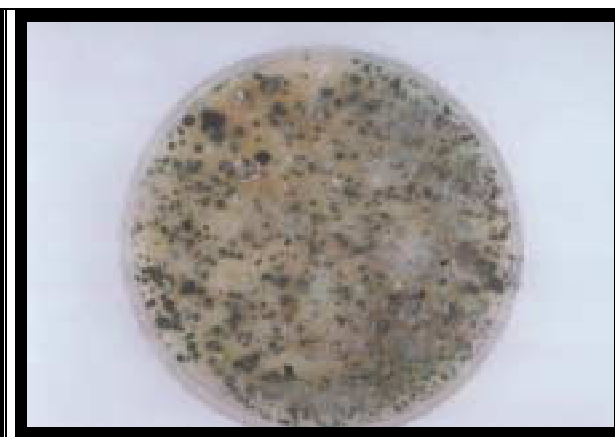
Thousands of A. fumigatus particles collected on Petri dish (8 cm diameter) from 100L of air aspirated 50m behind the turning machine
