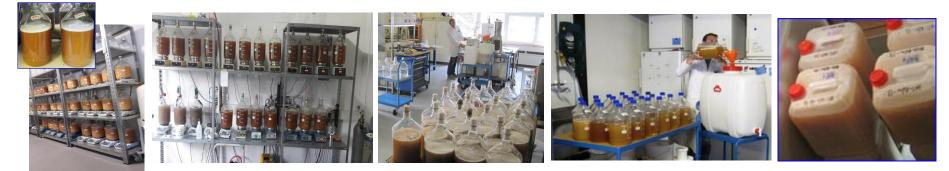
The micro-organisms are discharged directly into the digester, and for the soil / groundwater decontamination and wastewater treatment they are periodically suspended and / or multiplied on site for 24-48 hours in aerated cubitainers of 1-2 m3 (for WWTPs) and 1-20 m3 (for soil/groundwater).
