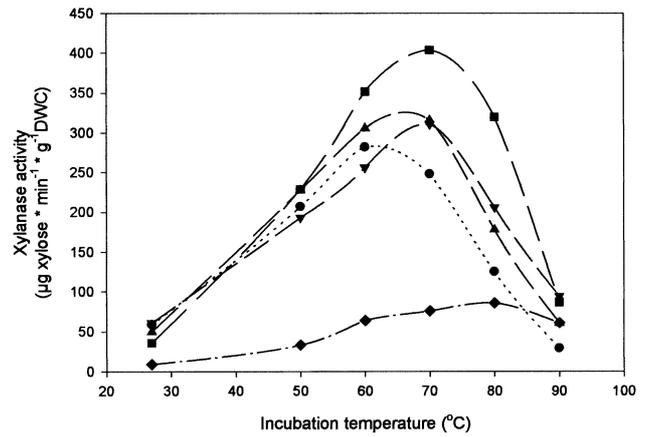
Fig. 5. Optimal temperature of xylanases in function of the localization of the compost samples in the trench. Xylanase activity measured at pH 6. Before turning: surface (.....), border (—■—) and centre (—◆—). Just after turning: border (—▲—) and ...●... centre (—▼—). Average of 3 to 4 samples. DWC – dry weight compost.
