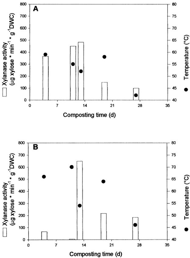
Fig. 4. Effect of composting time on xylanase activity at the border (A) and in the centre (B) of a trench. Compost samples were taken the same day, in different compost batches, just after turning of the trench. Xylanase activity was measured at 70°C and pH 6. ● mean temperature of the zone, □ xylanase activity. DWC – dry weight compost.
