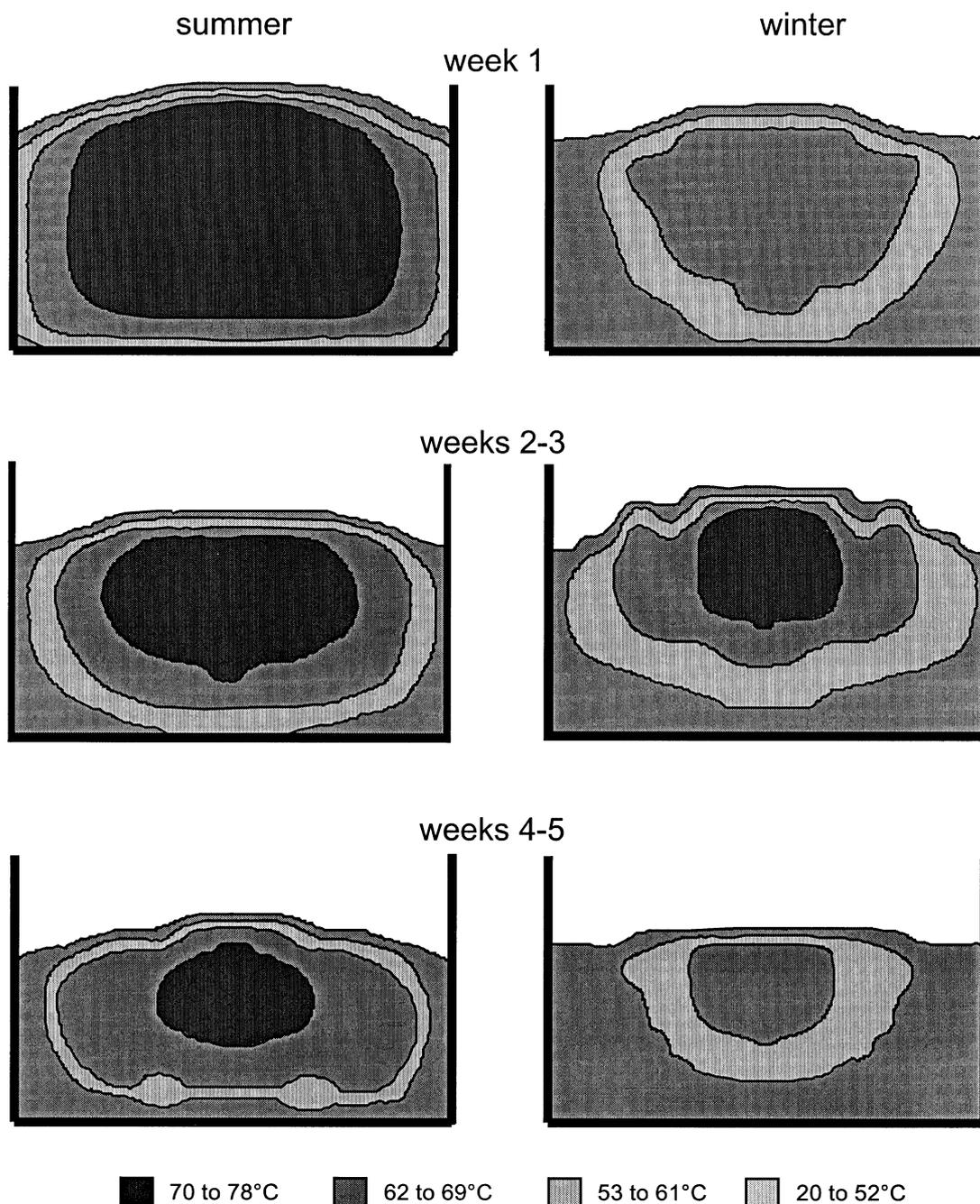
Fig. 3. Isotherms of three cross-sectional cuts showing the thermostratification evolution of summer and winter material. Average isotherms were obtained from 3 to 8 independent measurements.
