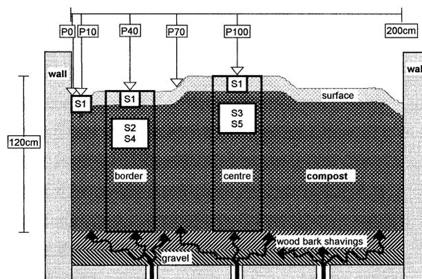
Fig. 1. Cross-section through a trench, filled with compost, showing the five different sampling points (before turning – S1 (surface), S2 (border), S3 (centre) and just after turning – S4 (border), S5 (centre)). The positions of the five vertical temperature profiles are also indicated (P0 to P100).
